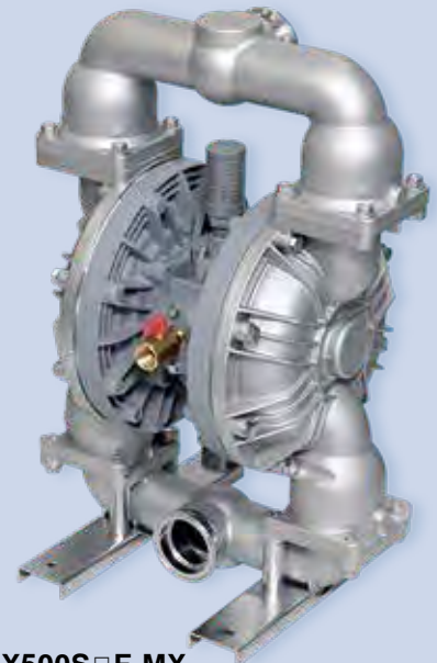
TC-X500S □ F-MX FDA Type Electro Polished SUS Pump. 2½" Sanitary Flange Connections. 520 L/min Max Flow Rate. (PTFE Diaphragms) 8mm Max Solids Size.
